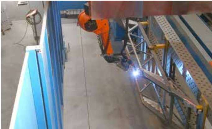
Photo 3: Another compact robot system welds elements for basket mast carriers and various small parts.
