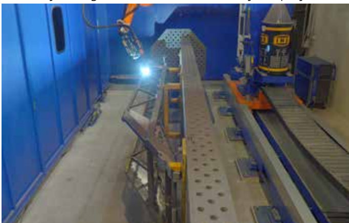
Photo 4: The workpiece is mounted between two vertically arranged faceplates.
