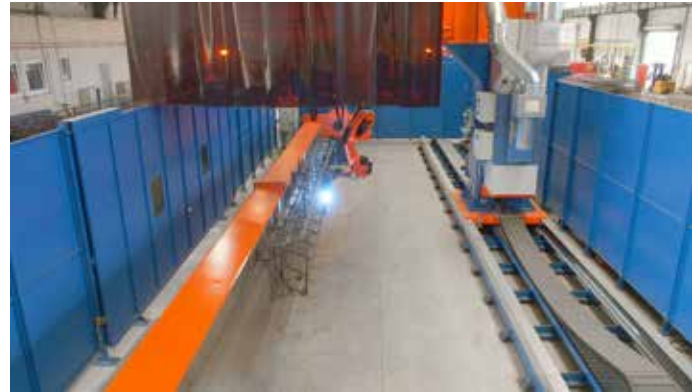
Photo 2: The robot has a greatly expanded working space as it is mounted overhead on a floor-mounted linear track with vertical and horizontal stroke.
