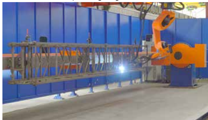
Photo 1: Two identical robot systems weld aerial ladder elements for fire brigade lifting vehicles.
