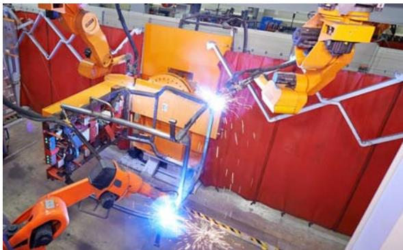
The workpiece positioners – equipped with a changing device— position the cabs optimally for welding every time.
