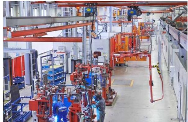
The complex cab-welding production line is more than 70 meters long and comprises a total of twelve stations.
