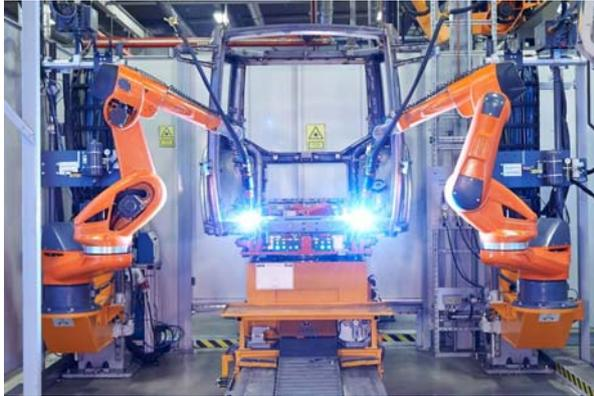
After pre-tacking in the manual stations, the 7-axis robots weld the cabs in automated systems.
