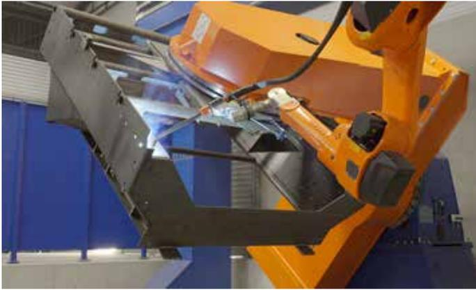
Photo 3: The workpiece positioner brings the grate trough into the perfect position for welding.
