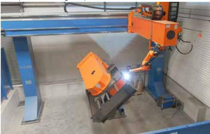
Photo 4: The robot is mounted in overhead position on an overhead-mounted linear track with vertical and horizontal stroke.
