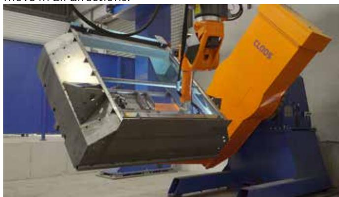
Photo 1: The new robot system weld grate troughs for waste incineration systems.
