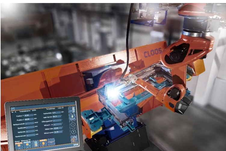
Photo 2 and 3: The C-Gate IoT Platform offers comprehensive monitoring of QIROX robotic systems and QINEO welding machines.
