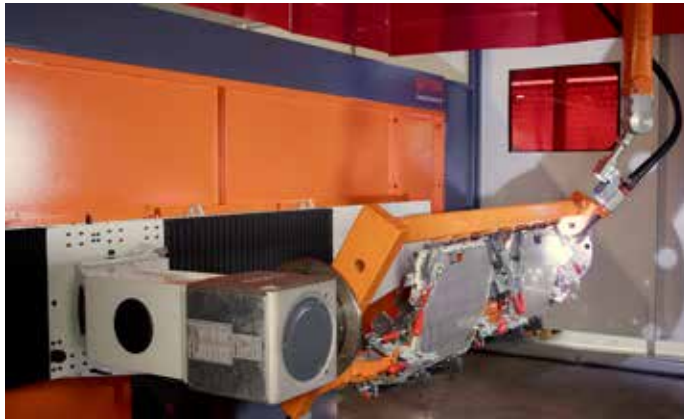
Photo 3: Among other things, multi-cycles welds side rails of the aluminium transport basket with the robot system.
