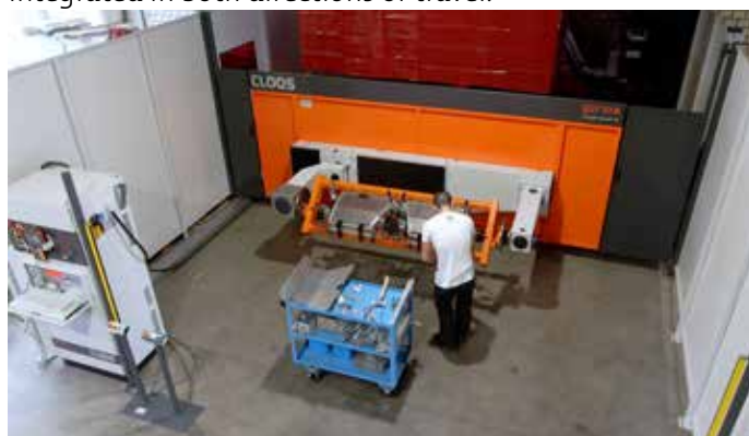
Photo 1: The two-station design allows loading on one side while the robot welds at the other side.
