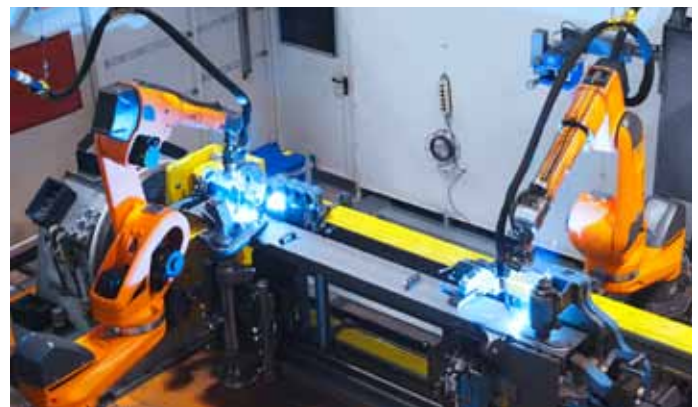
Photo 4: Linde Material Handling does not only use manual welding machines but also a multitude of robot welding systems.
