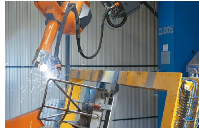
Picture above: Previously, one MAP employee used to weld 150 of these small parts per shift. Today, the welding robot in the compact system manages 350 parts per shift.
