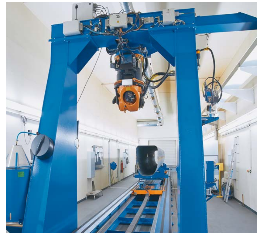
Picture above: The telescopic mobile crane booms are welded using laser-MIG/MAG hybrid technology: Manitowoc has stopped all submerged arc welding and thereby saved EUR 20,0000 annually on additional material and powder only.
