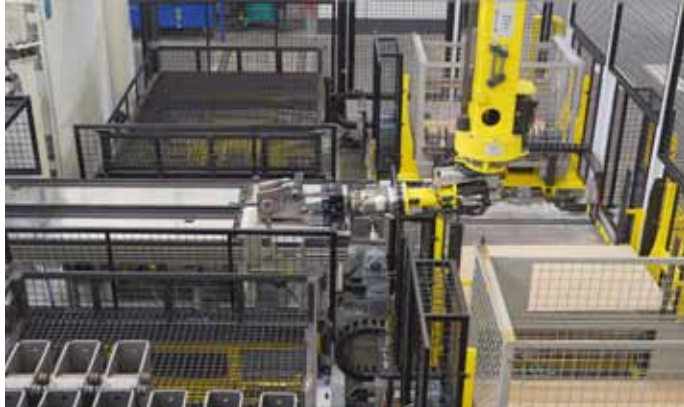
Photo 4: After the welding process, a robot automatically unloads the finished components.
