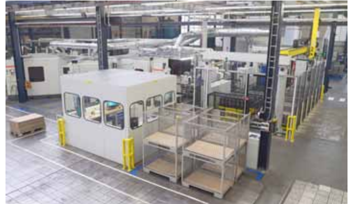
Photo 5: The system's welding fumes are extracted by means of a completely closed system.
