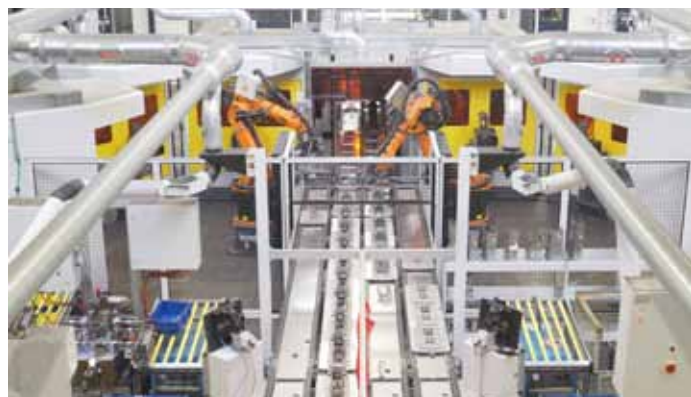
Photo 1: In the new robot system, the handling system and welding technology work hand in hand.
