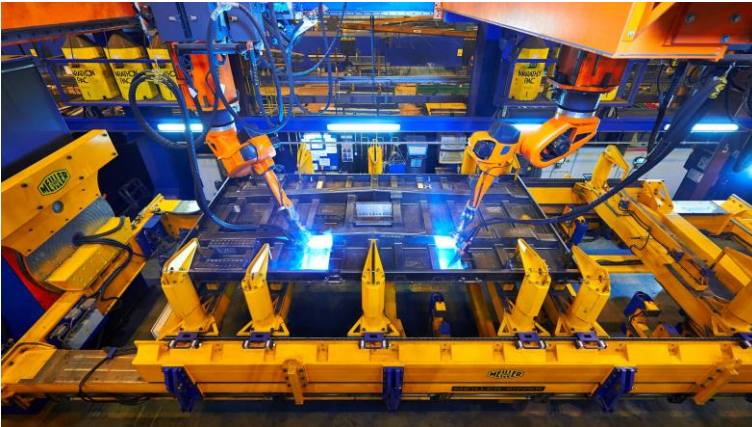
Photo 1: In the case of Tandem Weld two separate welding wires are fed and melted simultaneously in one molten pool.
