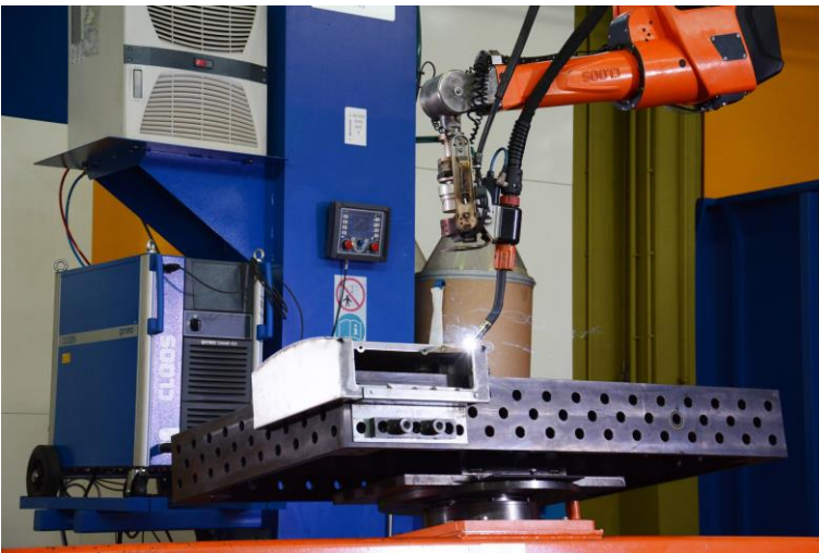
Photo 2: The increased deposition rate of the Cold Weld process results in enormous welding speeds particularly in the case of thin plates.
