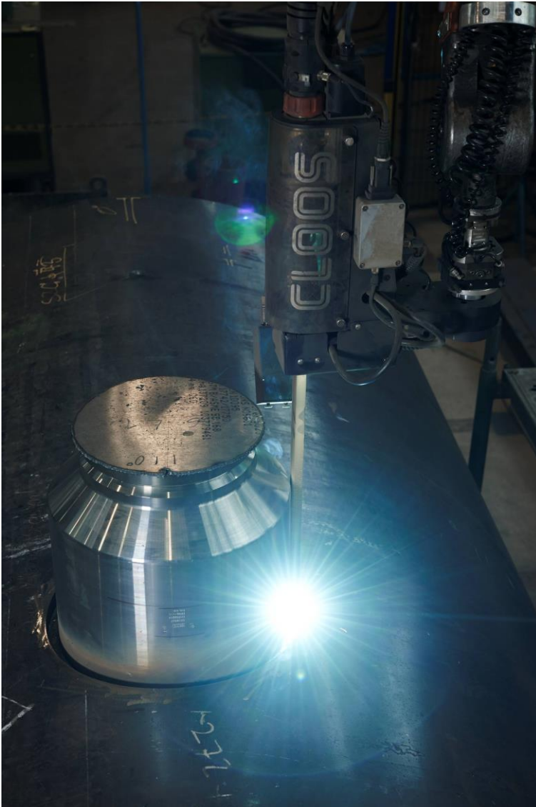
Photo 4: Shorter production times, considerably less material consumption and a high quality are the main characteristics of the narrow gap technology.
