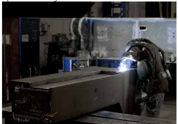
The new Cloos machines used during the welding of push-beams for crawler cranes.
