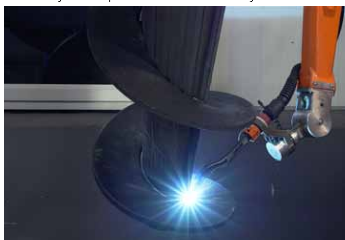
Photo 1: The robot welds the demanding radial seams of the screw compactor evenly and with consistently high quality.
