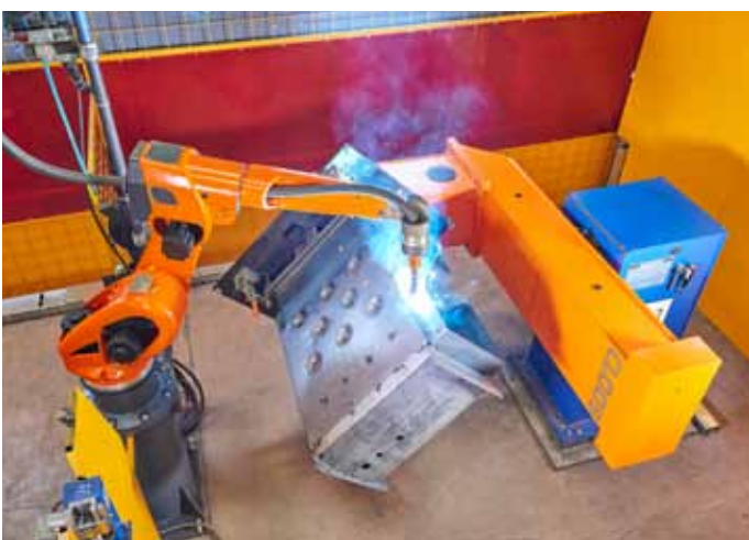
The WP-TS workpiece positioner always brings the boiler into the perfect position for welding.
