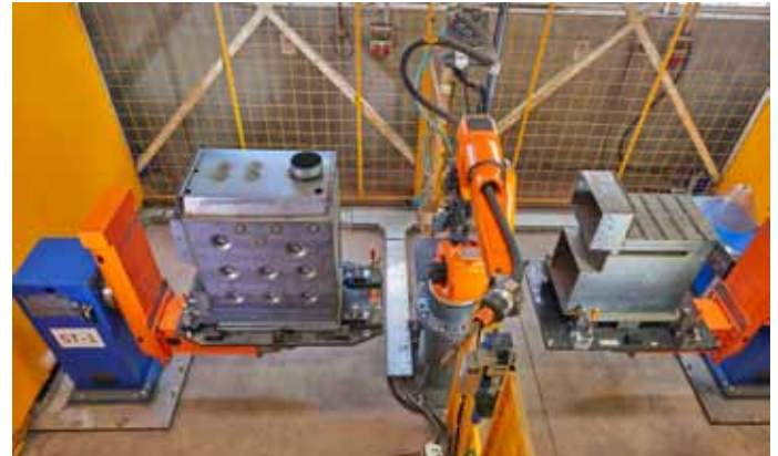
The two-station arrangement of both robot systems speeds the entire process run enormously.
