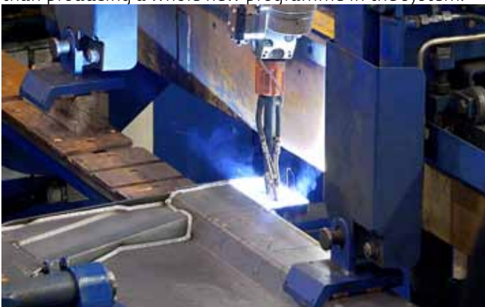
Photo 4: The torch is equipped with a laser sensor that measures the processing line online during welding.
