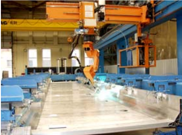
Modern aluminium assembly groups for the World market are welded on the 60m long robotic plant. With six internal and two external axes, the robot has optimum access to each required weld point.
