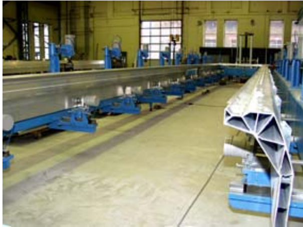
The peripheral equipments precisely position aluminium extrusion press profiles of up to 20m long for the robotic welding process.
