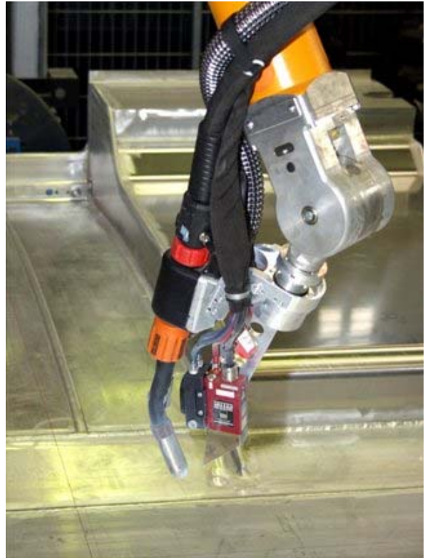
The laser sensor on the torch ensures optimum seam recognition and tracking and thus clean weld results.
