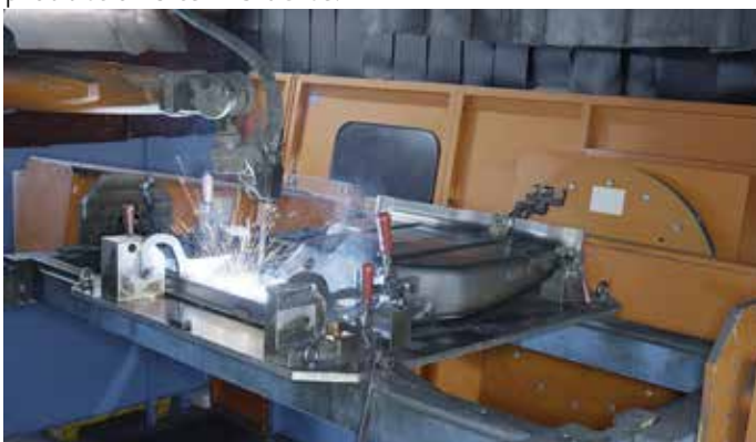
Photo 1: First, CLOOS robots weld the components.
