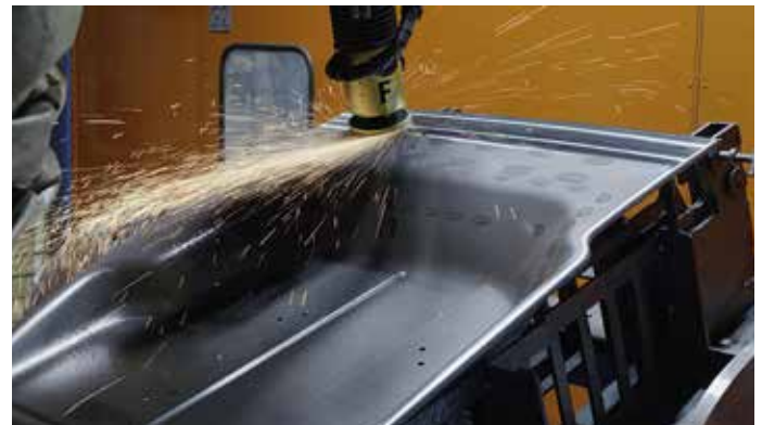
Photo 2: This is followed by the automatic grinding process.
