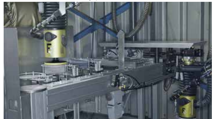
Photo 3: The tool changing system enables the use of various grinding applications.
