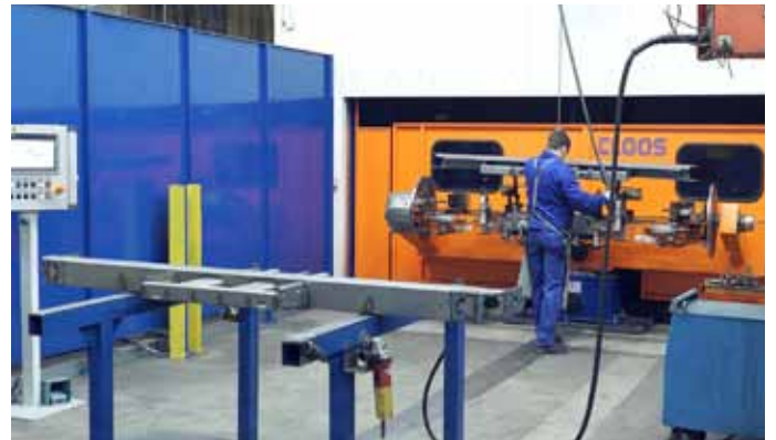
Photo 3: The two-station design allows the system's operator to load one station while the robots weld at the other.
