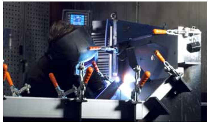
Photo 6: Welding a motor cover for a construction machine with QINEO Pulse.
