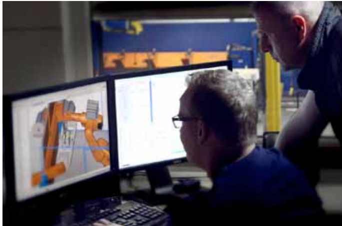
Photo 4: The offline programming of the robot systems is carried out using the CLOOS RoboPlan software.
