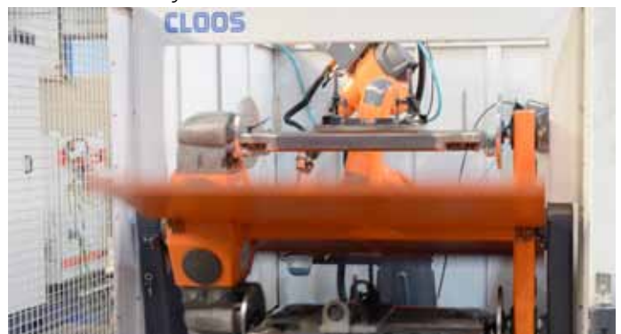
Photo 2: The compact cell has a 2-station workpiece positioner with vertical rotation.
