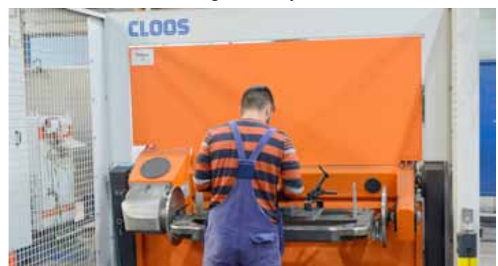
Photo 3: The 2-station design allows employees to load one station while the robot welds at the other.
