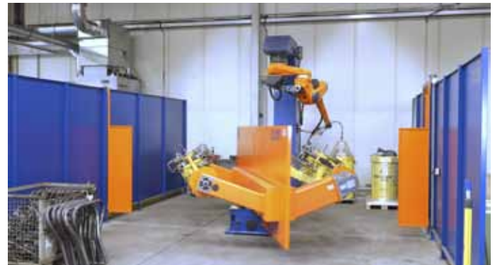
Photo 2: The station change of the WP-DH-TC two-station positioner is made by a horizontal rotation.
