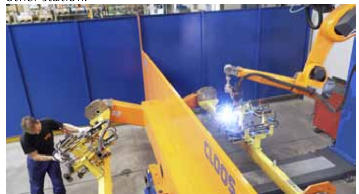
Photo 3: The 2-station design allows simultaneous welding and loading of the system.
