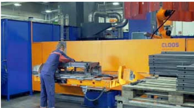
Photo 6: Because of the multi-station construction of the system, loading and unloading can take place parallel to the welding process.
