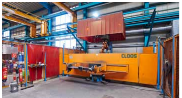
Photo 4: The positioner always places the workpiece in the optimum welding position.
