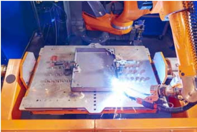
Photo 5: The large range of the seven-axis robot facilitates and accelerates the welding of the complex workpieces
