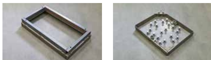
Photo 1+2: Manhole systems for cable distribution are welded on the two CLOOS robot systems.
