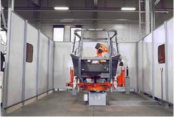
Photo 1: After the welding process, a CLOOS QIROX robot checks the quality of the finished tractor cabs.
