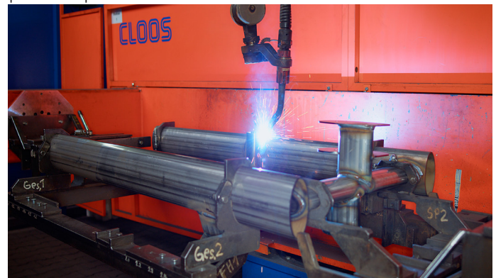
Photo 2: Around 70 percent of the components are now welded automatically.
