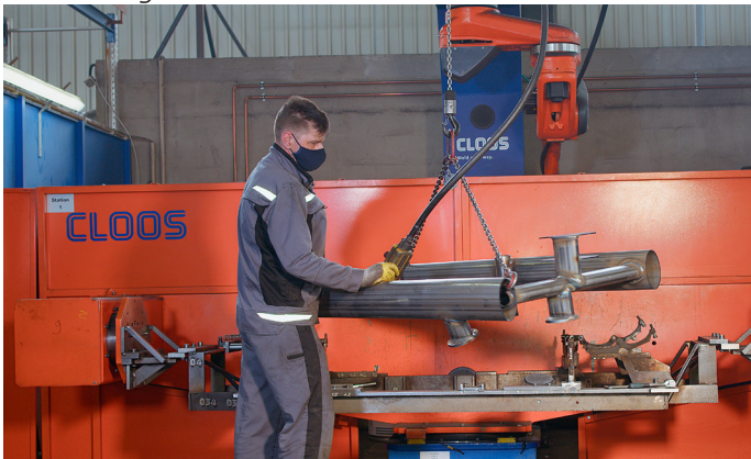
Photo 3: While the robot welds, the employee can load and unload the other station.
