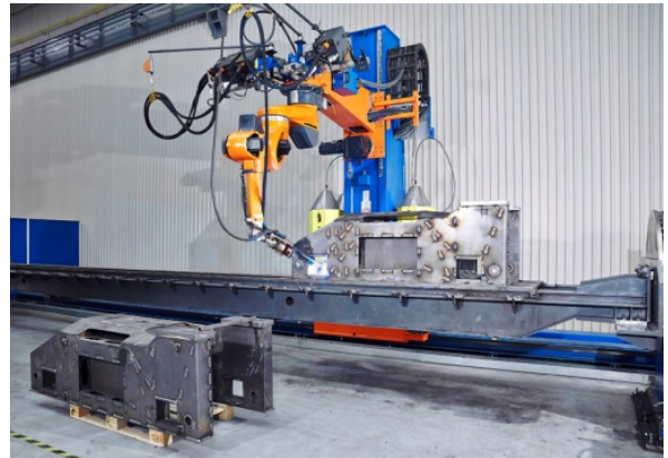
On this CLOOS robot equipment SSI Schäfer welds the up to 10 m long components of the new storage and retrieval device – the image shows a lifting truck weighing a good 600 kg. (Image: CLOOS)
