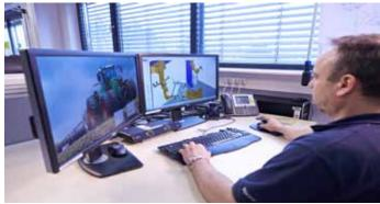
Offline programming with the Cloos RoboPlan software can be carried out even during production: an enormous time saving!
