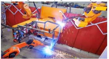
The workpiece positioners – equipped with a changing device – position the cabs optimally for welding every time.
