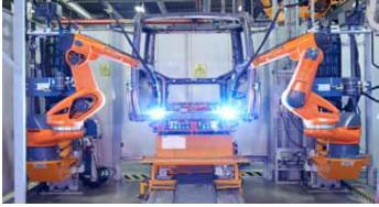
After pre-tacking in the manual stations, the 7-axis robots weld the cabs in automated systems.
