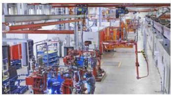
The complex cab-welding production line is more than 70 meters long and comprises a total of twelve stations.
