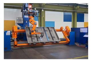
The turn/tilt positioner always positions the complex workpiece perfectly for welding.
