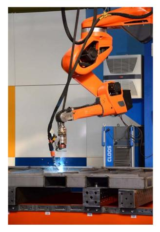
The increased deposition rate of the Cold Weld process results in enormous welding speeds in the case of thin plates.
