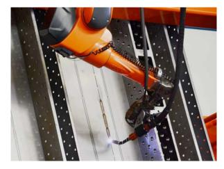
The reach of the 7-axis robot means that it can be easily guided around corners or into niches.
