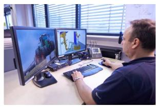
Offline programming with the Cloos RoboPlan software can be carried out even during production: an enormous time saving!
