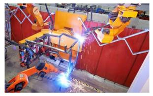
The workpiece positioners – equipped with a changing device  $\neg$  – position the cabs optimally for welding every time.
