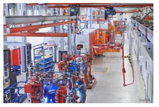
The complex cab-welding production line is more than 70 meters long and comprises a total of twelve stations.
