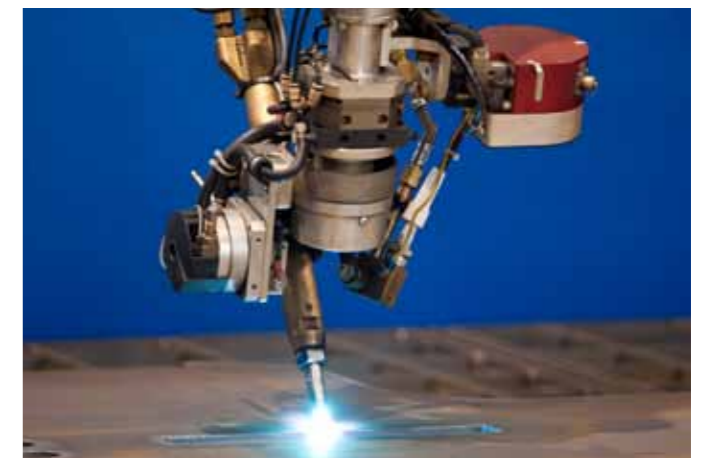
Another special feature: The automatic torch ignition with pre-ignition is a joint development by CLOOS and voestalpine.
