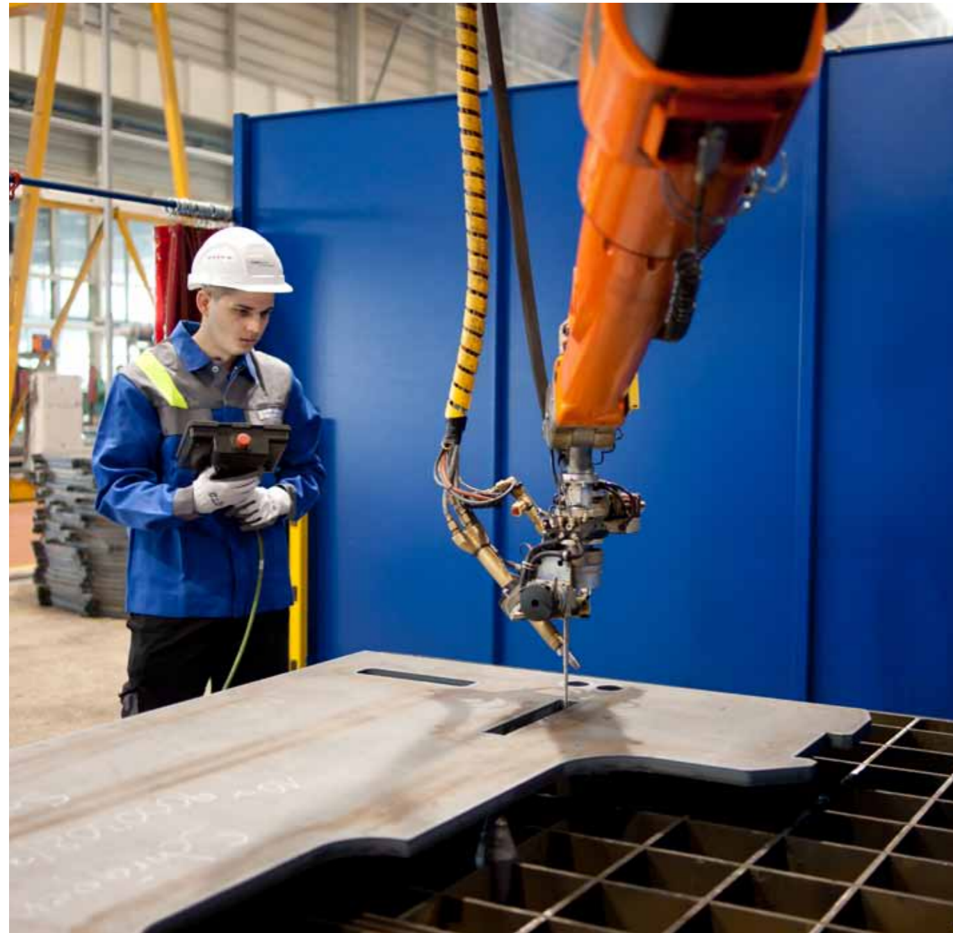
The robot cutting system consists of two stations and has a laser sensor with an additional tracer pin. While the robot is chamfering the blanks on one side of the table, the other side can be reloaded.
