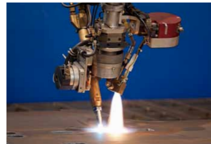
Another special feature: The automatic torch ignition with pre-ignition is a joint development by CLOOS and voestalpine.
