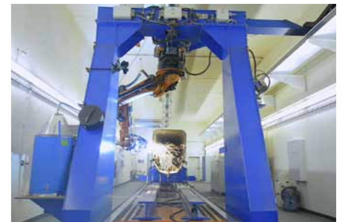
By hand, each hole took 15 min. The laser produces up to 30 holes in the same time.
