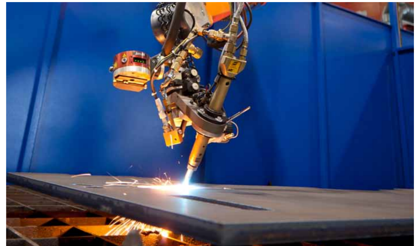
The robot uses a laser sensor to measure the precise position of the component to be machined. After that, the controller calculates the correct movement data for the robot and then cuts the blank out precisely. Then the station is released for workpiece removal and then reloading.
