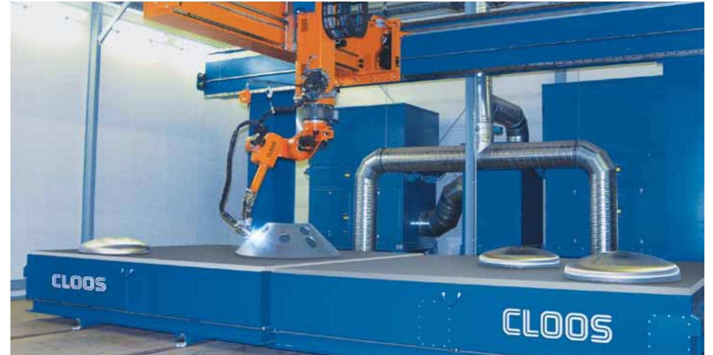
The robotic system consists of an 8 m long and 3 m wide gantry with a lifting height of 1 m. Here the robot type QRC-350 places the holes and contours in the conical head of the stainless steel container.
