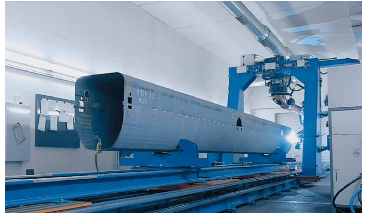
A mobile crane's booms comprise of a main element and up to 6 six telescopic sections, each of which can measure up to 14 m. The lower half is made of a thicker plate than the upper half. High-strength fine-graded steel with material thickness from 4 to 15 mm are used to produce the boom sections.
