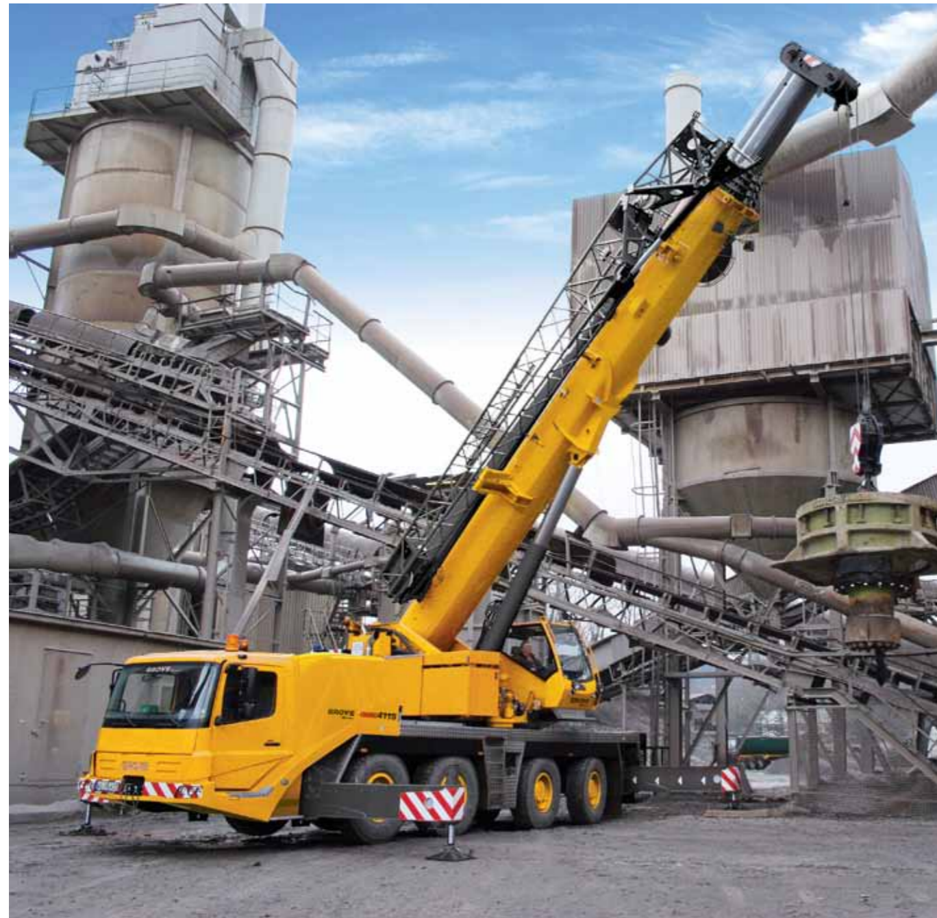
The Grove GMK4115 mobile telescoping crane with a max. capacity of 100 t, 11.3 m boom length and a boom angle of -1.5° to max. +82°.
