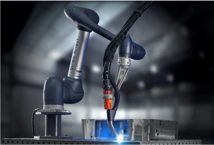
Photo 1: The new QINEO ArcBoT offers an easy entry into the world of automated welding.
