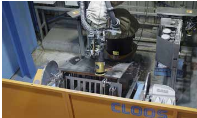
Photo 4: The robot also takes care of the fine grinding.
